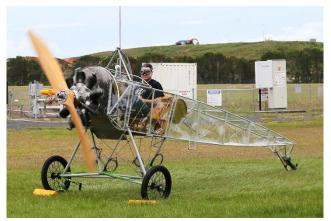
Running the CAMS rotary for the 1st time, fitted to E.III
