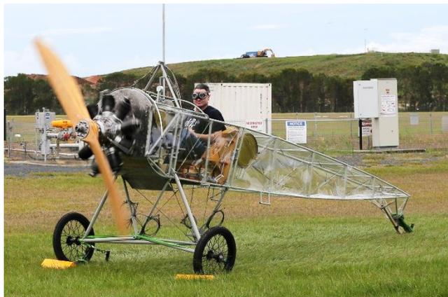
*Running the CAMS rotary for the 1<sup>st</sup> time, fitted to E.III*
